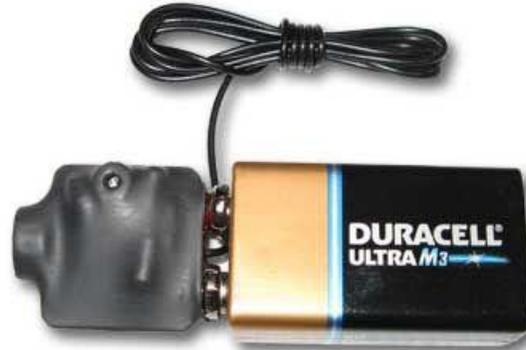
This is a medium-powered device that can pick up conversations/sounds within a 10 meter radius and transmit them to a dedicated VHF receiver or FM radio to a distance of up to 600 meters with good clarity. It is extremely simple to operate - just turn it on, tune it in, and you're away!
